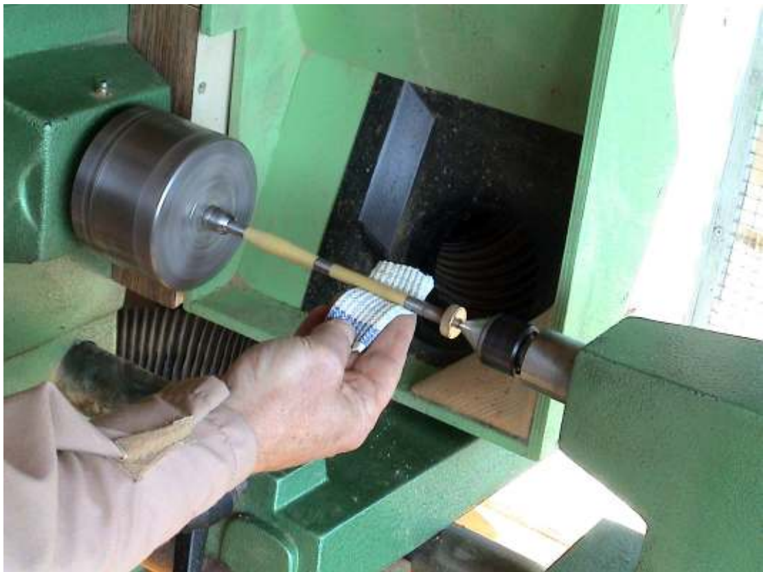
Various images showing a reasonably safe way to hold abrasive and woven fabric.
